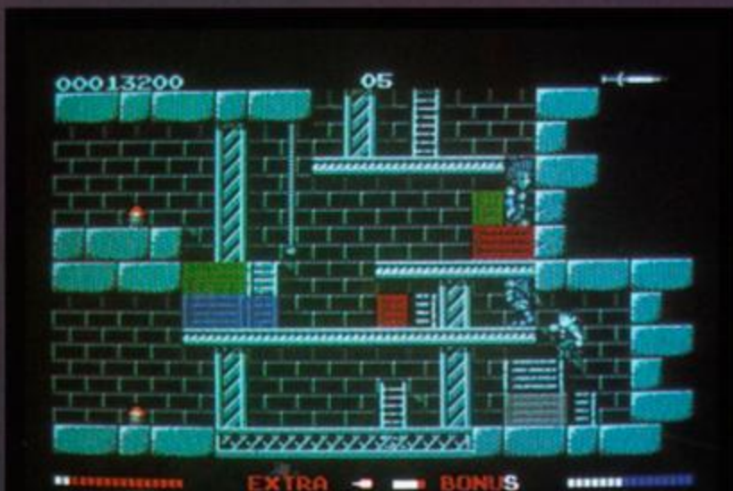
● Switchblade , technically, is done in the four-colour mode, but try counting the number in this screen shot! The programmers have used standard split-screen jiggery-pokery and the additional console hardware to 'cheat' on a grand scale.
