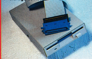
The 3.5 in. disk drive allows the CPC to transfer data between other computers, and is useful as a storage device.
