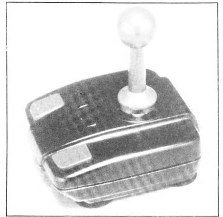
• Joysticks: OK for games, but not much good for graphics unless you have an analogue version – and a computer which can handle it.
