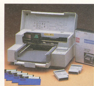
• Ink-jet printers fall mid-way between dot-matrix and laser printers in price and quality
