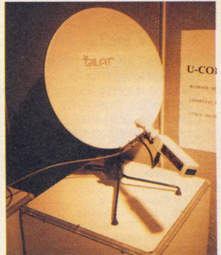
• Gilat's U-Cord system – a receive-only terminal for data communications able to incorporate different satellites and antenna diameters and capable of handling up to 112Kb per second of data. Prices for this remote terminal start at £800.
