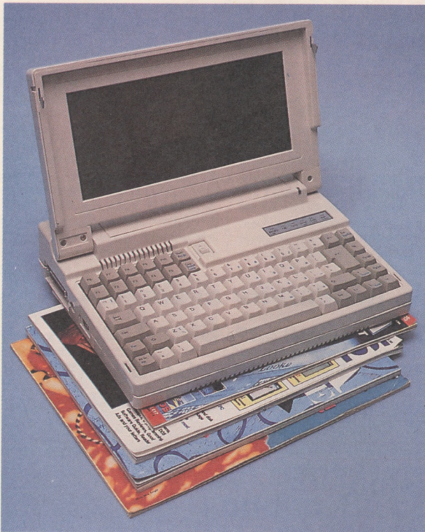
• (Left) The Protocol is no bigger than an A4 glossy magazine. It's light and very portable. There's a backlit LCD screen which provides a full 80 x 25 CGA text and graphics display and combined with the fully-featured, sculpted keyboard the machine is ideal for writers and journalists on the move, as well as salesman and executives
