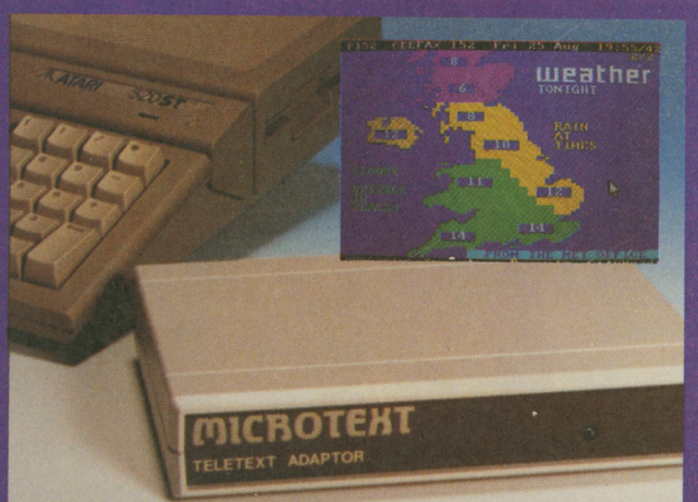
• Microtext's teletext adaptor lets the ST page the Oracle, 4tel, Ceefax...
