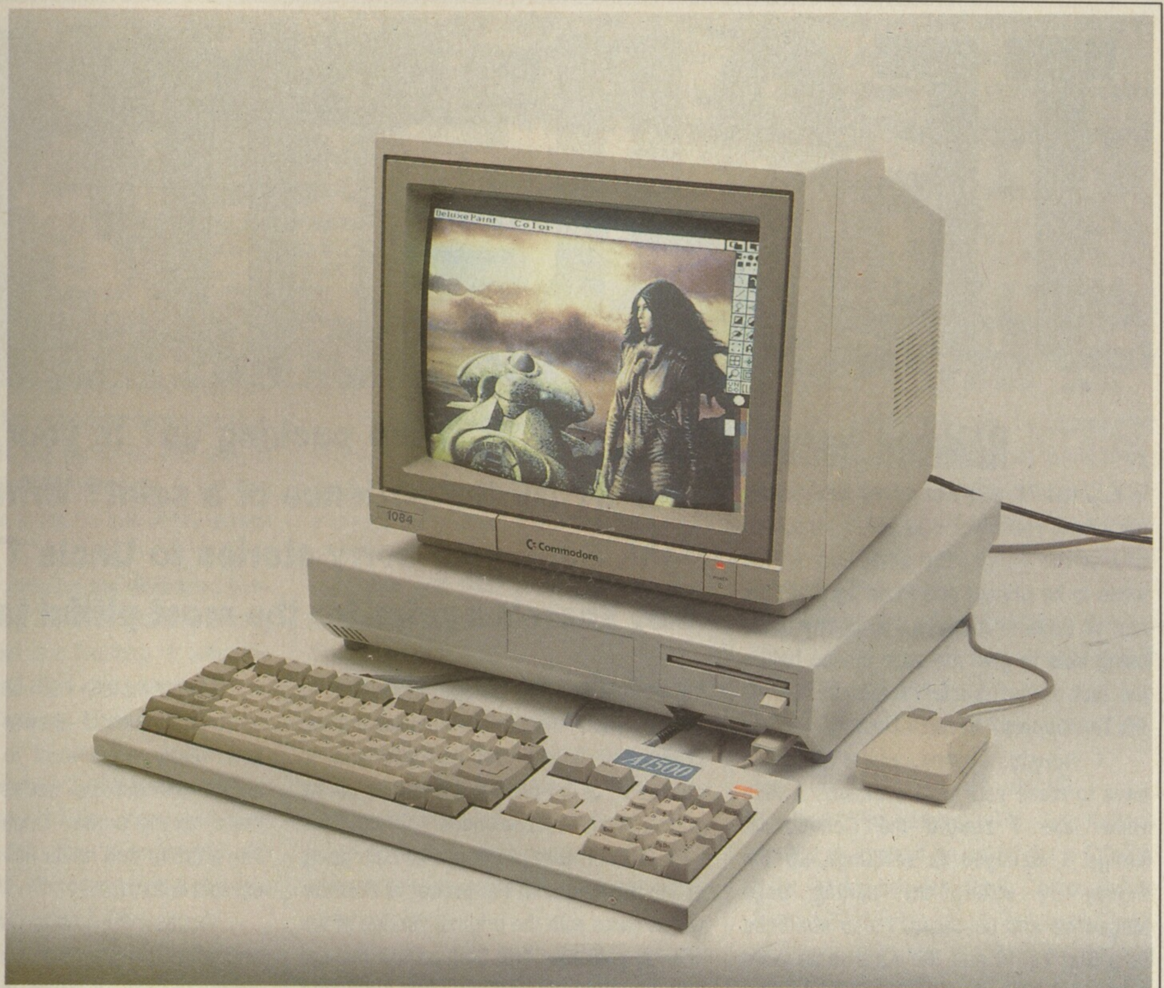
• The A1500 adds a smart new case and expansion ports to an A500.
