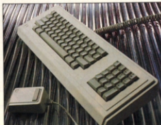
Lisa's keyboard looks ordinary but it's different: every key can be programmed individually.
