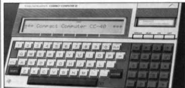
Business and technical users of TI's new CC-40 will be able to plug in software packages on 128K ROMs.
