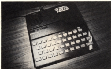
BOXING CLEVER — The Fuller Box is a neat unit which attaches to the rear of the Spectrum. It tidies up some of the Spectrum's shortcomings by providing a joystick controller, bleep amplifier and more reliable cassette interface. The joystick controller is port-mapped at 127 and will accept joysticks from Atari and Commodore. These will control all the games from Imagine. The bleep amplifier amplifies the Spectrum bleeps under a volume control and the cassette interface is claimed to eliminate the problems often encountered saving programs when mic and ear jacks are in at the same time. The Fuller Box costs £29.95 plus 80p p&p. Fuller can be contacted on 051-236-6109.
