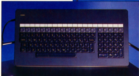
Top — The uncluttered rear view showing the practicality of recessed easy-access card slots. Left — Clear easy to use keyboard highlighting the large numeric keypad on the right and the row of 20 function keys.
