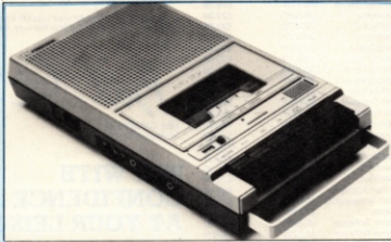
SOCKET TO 'EM — Ferguson claims that this 'champagne presentation model' 3127 cassette recorder comes with computer compatibility. What this means is the recorder has a five-pin DIN socket and a remote control socket. The company says it was designed to work with all makes of micro (except of course the idiosyncratic Commodore machines), and it should start appearing in the shops within the next couple of weeks at a cost of around £24.
