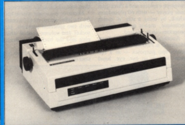
PRINTER-PLODDER — This solid-looking beast is the latest daisy-wheel printer from X-Data. It costs £695. The EXP550 can print bi-directionally and handles paper up to 17in wide. Standard interfaces are the RS232C and Centronics. Unfortunately the printer is capable of only a meagre 16cps — slow enough for you to take lunch while a substantial document is printed. If you want a cheap typewriter-quality printer for an occasional letter, it could be worth looking at. Tel (0753) 723331.
