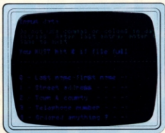
File Handling records are fixed to name, two-line address, phone and 'ordered anything' fields.
