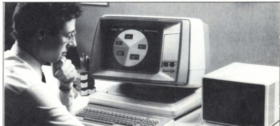
The eight-colour ET2200 with primary colours driven by three 128K processors.
