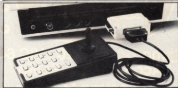
DELTA BELTER — If you play games on the BBC micro you can, quite literally, bash the living daylight out of your keyboard. This Delta 14 handset is designed to relieve the keyboard of such punishment. It is an adaptation of the handset used for the Database video game and costs £10.95. An optional adaptor box costs £13.95 and allows you to use all 14 keys, which can be configured to work with the more complicated games. The Delta 14 is manufactured by Voltmace (0462-894410), which is currently negotiating with software companies to produce options in future products that make use of the handset's capabilities.
