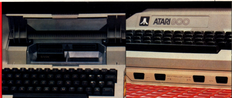
Above left, the Atari's cartridge slots. At the front are two slots which take the Basic or other language cartridges, plus games or utilities. At the rear are four slots for the 10K operating system pack, and additional memory. On the right, the interfaces at the front are for game paddles and joysticks.
