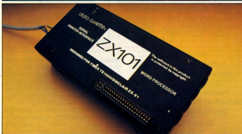
Top: The GP100AS — no nonsense printing at a good price. Above: Firmware and RS232 inter face combined.
