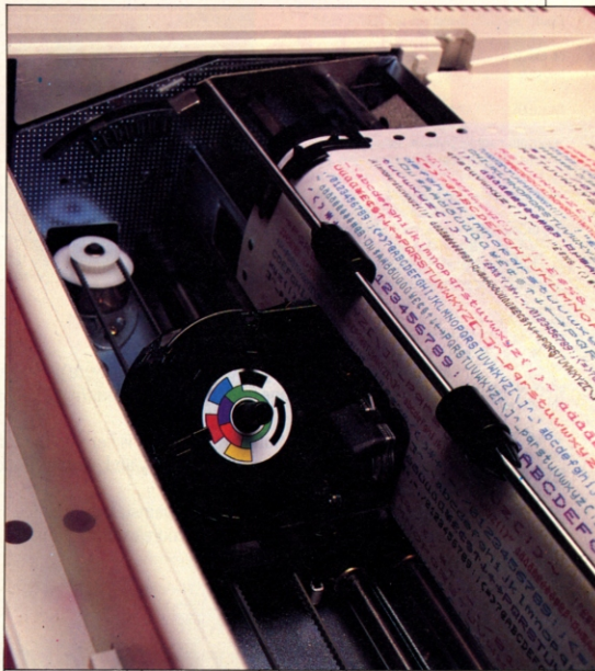
Colour close-up. The GP-700A's unusual print mechanism is a change from the usual wire-plan hammer. See box (left) for details of how this printer gets dots onto paper.
