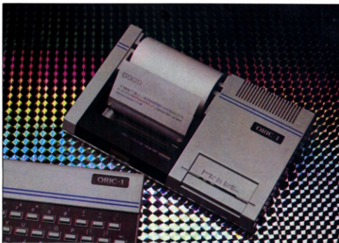
The four colours (red, blue, green and black) are in small cartridges which are placed into a barrel type pen holder on the printer. To achieve printing, the paper is moved up and down as well as sideways. When printing is in progress, a small lever on the bottom of the barrel is moved forward and this moves the whole barrel forward as well. The colours are changed by the barrel moving to the left of the printer where a small metal lever 'clicks' the barrel over to the required colour. The ink cartridges are good for 250 meters (825 feet).
