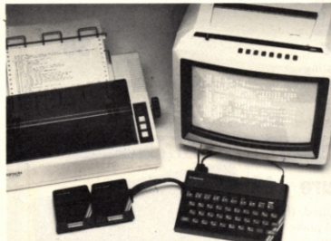
The Microdrive Interface 1 includes an RS232 interface allowing connection with peripherals such as high quality printers.
