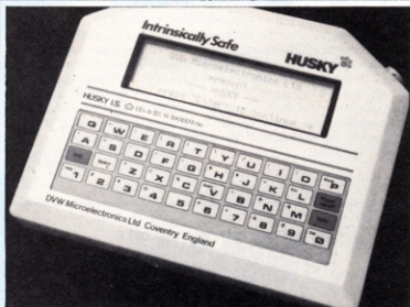
WARN AND HUSKY — DVM Microelectronics has repackaged its Husky portable to make it suitable for anyone using a micro in what it describes as 'flammable or explosive atmospheres'. The new model is known as the Husky 15 (Intrinsically Safe). The Z80-based machine with 128 character LCD will sell from £2,099 for a 16K version to £3,144 for the 144K version. DVM is on Coventry (0203) 668181.
