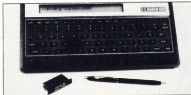
HP-75C and one of the cartridges — three can be installed at once.
