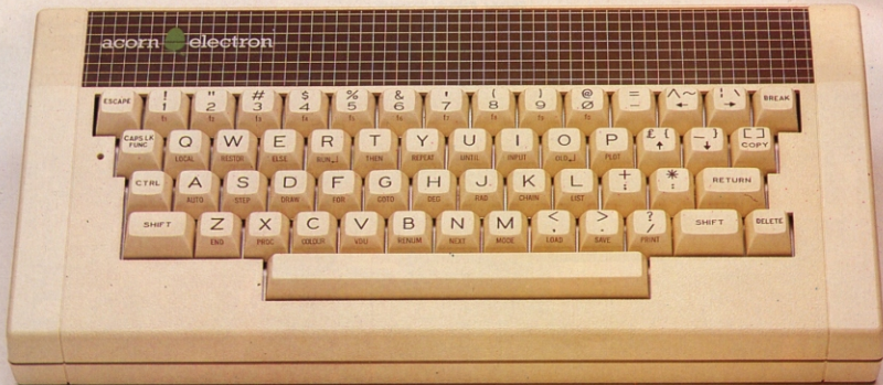
Above — Ten programmable function keys are available and they work just like those on the BBC.
