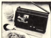
Sinclair's flat-screen TV uses a single integrated circuit chip to perform the majority of signal processing functions. The £79.95 Zin TV is the first television to have all such functions controlled by a single chip.
