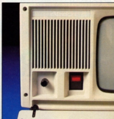
Top: The Miracle's 386K disk drives. Below: External controls are for brightness and on/off
