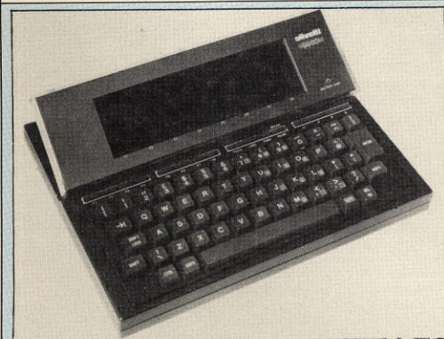
HANDY PORTABLE — Olivetti has joined the ranks of Tandy and NEC with its own portable called the M10. About the size of an A4 sheet of paper the M10 has a pop-up, 40 x 8 display screen, query keyboard and 32K ROM which contains the Basic interpreter, text editor, address book and diary. Two versions of the machine will be available — an 8K model at £499 or 24K at £699. You can get your first glimpse of the M10 plus its add-ons at Compec '83, Olympia London.
