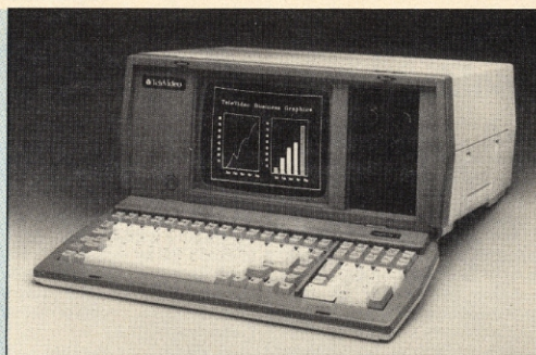
PORTABLE NETWORKING — Televideo has moved into go-anywhere multi-user computing with its new TelePorter portable machine. The machine weighs 25lbs and plugs into the company's networking system. It costs £1,351.25 and comes with a Z80 processor, 64K RAM, one 5 1/4 in disk drive, a SuperMouse for graphics applications and two RS232 ports. Free software that comes with the machine includes a word processing package, financial spreadsheet, TeleChart, and the GSX-80 graphics systems extension. Contact Encotel Systems Ltd, 01-686 9687.
