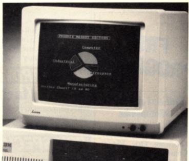
SCREEN TEST — Emco has launched a colour monitor, the Luxor, as an alternative to IBM's PC monitor. It has a 14in screen, anti-glare glass, a high resolution of 820 x 640 and is surrounded by a tough metal case. With a simple chip change, the monitor is compatible with most micros. It will be sold through IBM dealers at a price of £540. Further information from Emco (01-737 3333).
