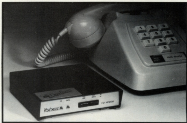
The Buzzbox from Scicon is a hardwired modem offering both originate and auto-answer for £70.
