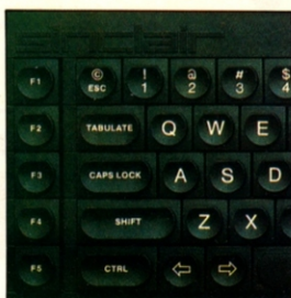
Sinclair has dispensed with the penny-pinching keyboards of the ZX days. This one still uses a touch-sensitive membrane, but the keys mimic full-travel and the QL registers a 'click' to provide some feedback.
