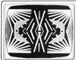
The mirror option can be used to give vertical, horizontal, diagonal or 4-way reflections.
