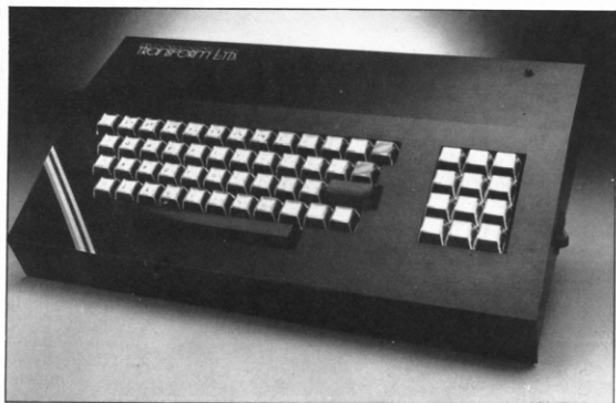
The Transform is a metal cased keyboard, with plastic topped keys which allow you to interchange the inscriptions. The Transform also boasts a separate numeric keypad, for those with an interest in accounting.
