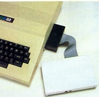
The sprite board plugs straight into the cartridge port of the Dragon. The TV now gets plugged into the board, and the signals all come from this, not the Dragon.
