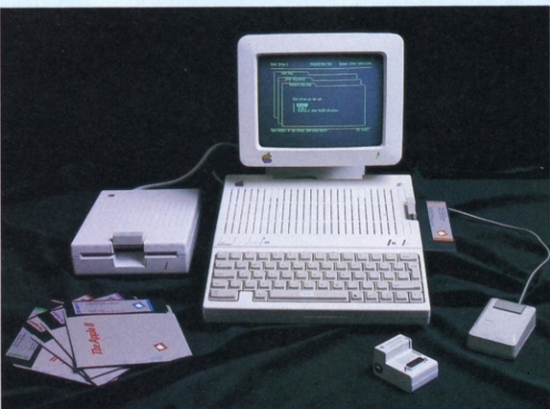
IIc complement: the monitor, second disk drive and mouse are optional extras.
