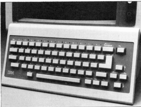
The PC jr's 62 colour-coded keys help users to follow the function and Alt key combinations.
