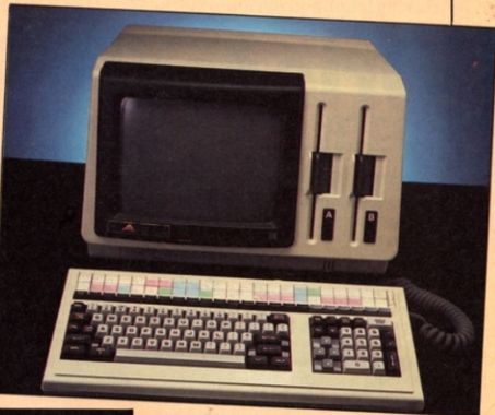
NEC APC: MS-DOS but little chance of taking an IBM floppy in its 5 1/4 drives.
