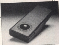
Heat-seeking mouse — infra-red connection and twin functions in a device that can be a mouse from one angle and a trackball from another.
