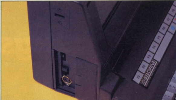
The on/off switch and power input socket are located on the left of the main unit. A battery power-pack is optional.
