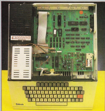
Above: Inside the Einstein — the speaker sits at the front of the 'chip board' facing the user. Below: The demonstration program shows off with sound and graphics.
