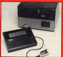
HUSKY BAR — The rugged Husky handheld portable is proving to be remarkably adaptable. Latest additions to its peripheral range are a bar code reader and printer. Software comes on ROM allowing it to converse in the popular UPC/EAN grocery code with input via an optical wand or the keyboard. The 8610 thermal bar-code printer prints out the bar-codes on to self-adhesive labels. Just the ticket for shopkeepers.
