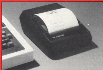
SMALL PHRY — BBC and Electron users can hook up this 40-column printer to their machines. At £113 the PhiPrint comes with a Centronics interface and cables, and can print in true descenders, lower case characters and underline. Other features include bit image graphics and character modes. It is sold by Phi Mag Systems (0326 76040).
