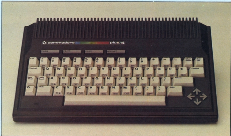
The keyboard is similar to that on the SX64 and the cursor keys are conveniently placed.
