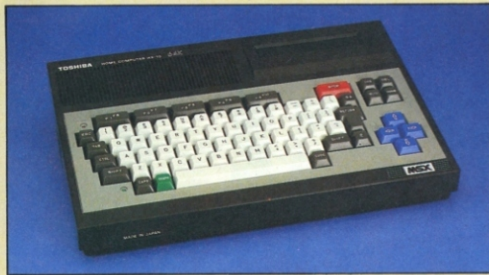
All the MSX machines will have a standard ROM cartridge socket. Power is automatically switched off while inserting a cartridge.
