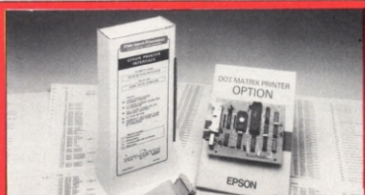
FIT TO PRINT — Sharp 700/800 micro users can link up to all Epson dot matrix printers with this E79 interface board. Main attractions are software compatibility and direct printing of all Sharp graphic characters. The 8,000 character buffer shouldn't come amiss, either. The device slots into the printer, comes with a 1.5 metre cable, and is available from main dealers. Details from Mills Harris on 024262-341.
