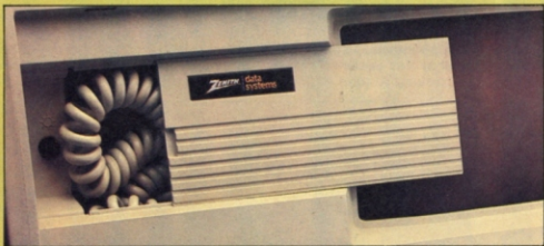
The keyboard cable and the controls for the screen are hidden behind a sliding panel.
