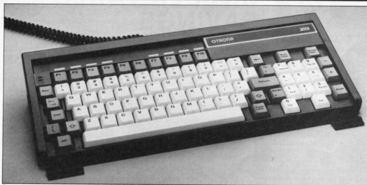
Even though the keyboard is a membrane type, it has a very high quality feel.
