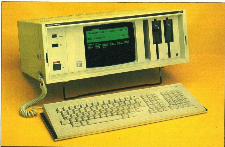
Once set up, the system's two 640K half-height disk drives are to the left, flanked by the keyboard cable's compartment.
