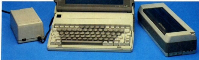
The DG1 is one of the first machines to use a full-size LCD display. Even though the keys appear smaller than usual, the keyboard is still high-quality.
