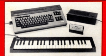
KEY FEATURE — The most distinctive of the MSX micros to arrive in the UK was launched last week by Yamaha. The CX5 combines the standard micro with an FM sound synthesiser, so that the array of ports at the back of the machine includes in and out sockets for MIDI (musical instrument digital interface) devices. With a small keyboard the CX5 costs £334; the larger keyboard (M1) to £614. A 96K RAM expansion costs £65, and various items of ROM software for musicians cost £36 each.
