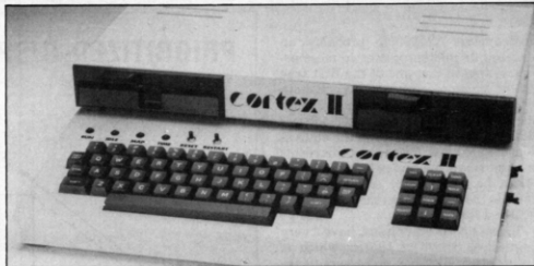
The dual disk drive is designed to sit neatly on top of the machine.
