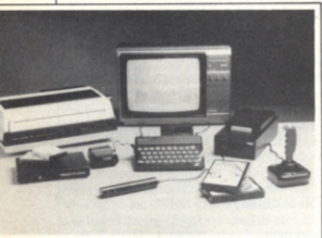
The Interface 2 allows you to use ROM cartridges and joysticks with the Spectrum.
