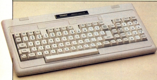
The keyboard doesn't wholly toe the IBMline: the function keys are across the top, rather than down the side.
