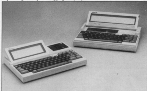
The Talbot Dialect 4 appears at first sight to be a cut down version of the Epson PX-8 (right). Obviously the display on the Talbot is half the size, so some software will not work. Programs stored on micro cassette will load however, which allows you to transfer text from one machine to the other. Unfortunately, the utility ROMs are not compatible, so you can't use Intex on a PX-8. But, Basic programs can be swapped between the two machines without too many problems.
