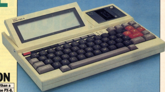
The keyboard on the PX-4 can be replaced by a dedicated type.
