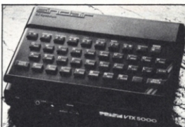
With Spectnet and the VTX5000 you can access on-line services in the UK and the US.
