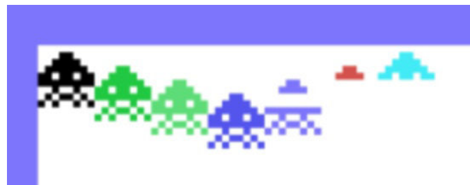
Figure 1 - TMS9918 displays only 4 sprites per scan line
