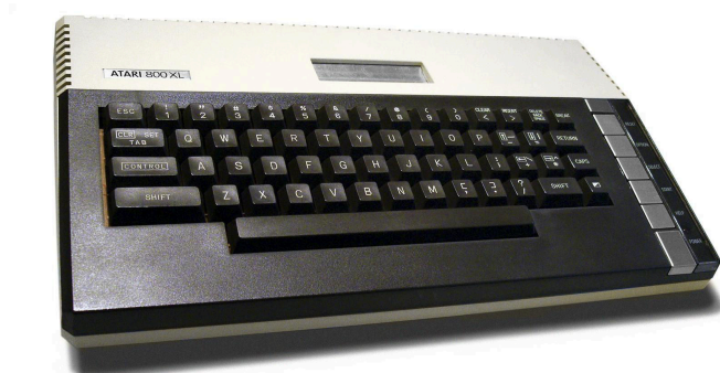
Figure 1: The Atari 800XL mounted the custom ANTIC, GTIA and POKEY chips to lighten the CPU from video and sound management.
