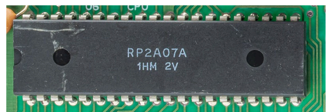
Fig. 8 - The CPU produced by Ricoh for the Famicom/NES, here PAL version (author: PantheraLeo1359531 - source: Wikimedia Commons)
